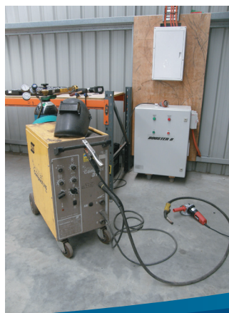
A Booster running a three phase Mig Welder
